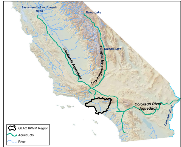
The primary sources of imported water supplies to the Region are the State Water Project, the Colorado River Aqueduct, and the Los Angeles Aqueduct.
